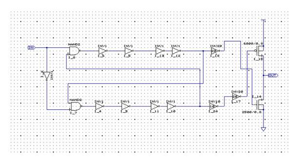
The RS flipflop sets the true and complement of the waveform. The inverters provide delays so that when the p – channel output transistor is ON the n – channel is OFF and vice-versa. A simple yet useful circuit.
