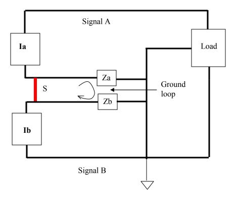
The short shown in red ( or thicker line) creates a ground loop. Any magnetic flux that couples in this loop will cause large currents to flow in the loop because of the low impedances of the ground lines. This can cause all sorts of problems including burnt out traces and severe noise.
